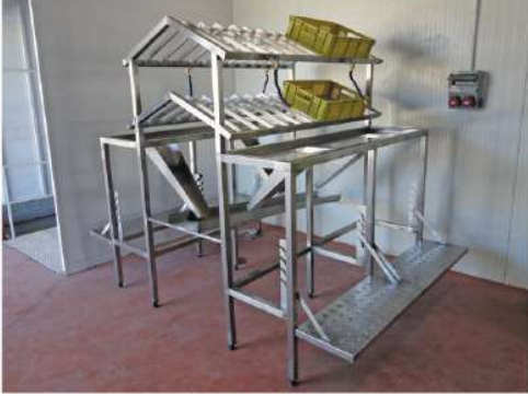
Kaşar Kurutma Arabası Kashar Cheese Drying Trolley (These are used for resting and transfer of kashar cheese after production)
